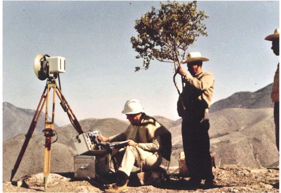
Fig. 8: To measure a distance between 100 m and 50 km, a DI50 was set up at each end-point and the distance calculated by measuring the transit time of the microwave radiation. The picture shows a DI50 being used in Mexico.
