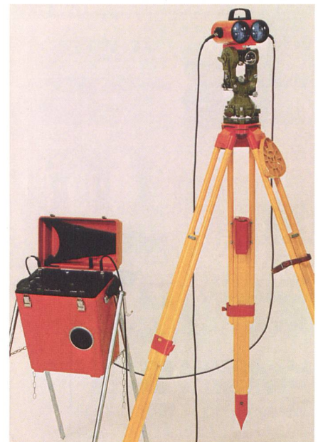
Fig. 9: The DISTOMAT DI10 on a T2 theodolite together with the control unit.
