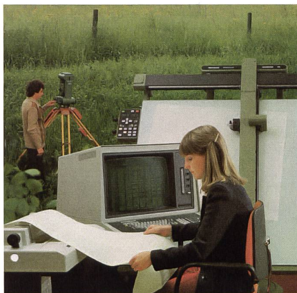
Fig. 13: The GEOMAP system. The screen was used to display the graphics. Top left a TC1 and to the right the plotting table are shown.
