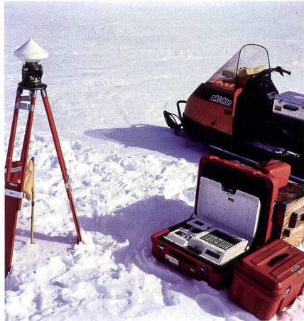
Fig. 14: The WM101 GPS surveying system "is an easily transportable piece of equipment weighing only 14.5 kilograms" – an extract from the advertising in 1984. Here shown on a 1991 Greenland expedition.
