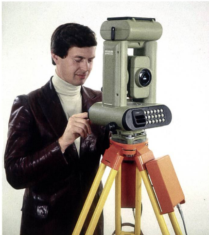
Fig. 12: The Wild TC1 was a fully automatic tachymeter with a cassette recorder for digital data storage.
