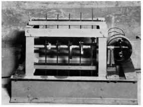
hammers of 500 grams each, lifted by cams and then dropped at intervals of about one-fifth of a second. 13 This weight and speed proved most suitable, although other laboratories built numerous alternatives.
