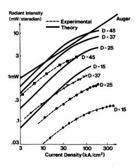
Fig.4: Light vs current showing saturation
