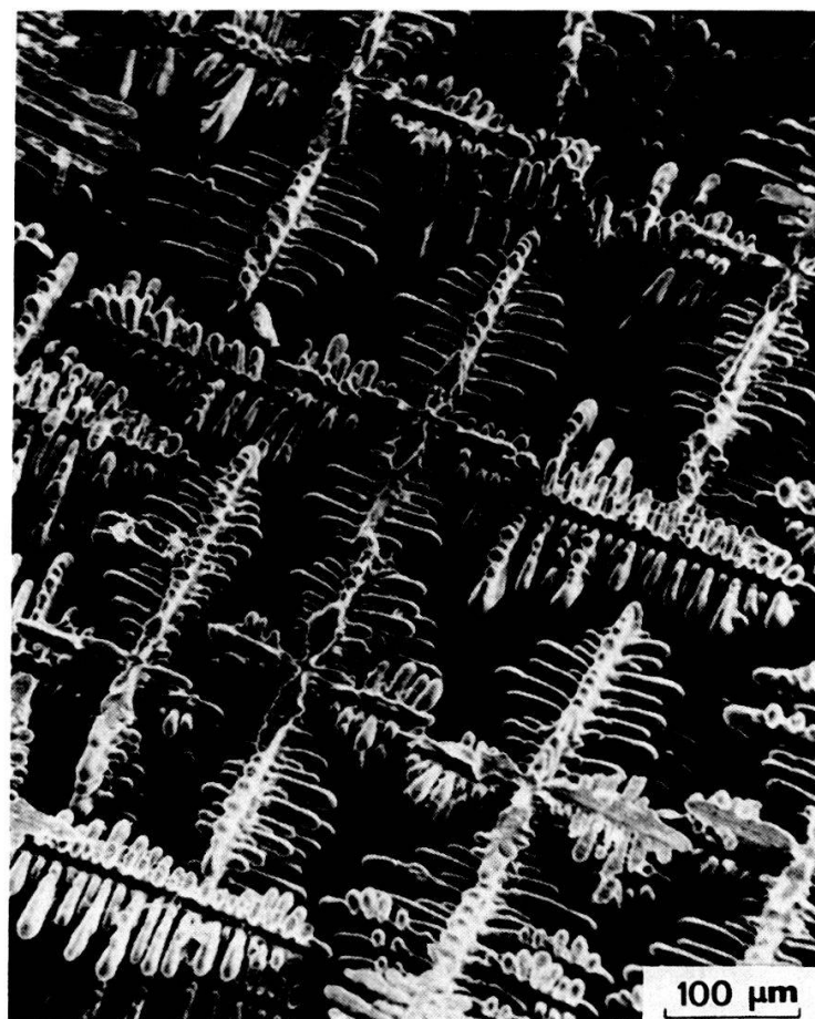
Figure 3 Co-dendrite during growth after eliminating the liquid phase.
