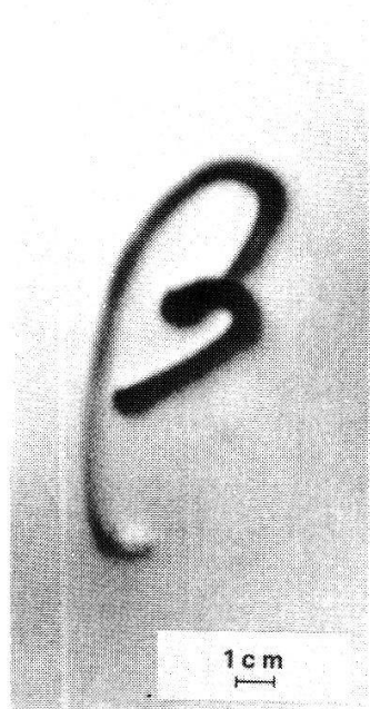
Figure 5 The effect of static charging on the suspension. The letter \beta has been written with a synthetic brush.
