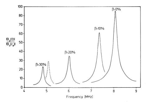
Figure 1 Resonance curves of the MAR for a model plasma with linear density oscillation profile and m = 1 for different maximum levels  $\beta$  of the density oscillation in percent of the undisturbed electron density. The dashed curve shows the approximate solution for  $\beta = 30\%$  where only N = 3 equations are considered in the system (21).
