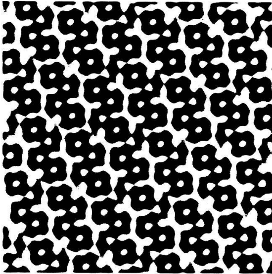
Figure 1: Quasiperiodic pattern calculated for k_c d \rightarrow 0 . The angles are \alpha_3 - \alpha_2 = \alpha_2 - \alpha_1 = 0.7 . The greyscale codes the deviation of the temporal average of the component of the magnetization perpendicular to the film from its thermal equilibrium value. Black means no deviation. Such an image would be expected in an experiment using Faraday rotation as a visualization technique.
