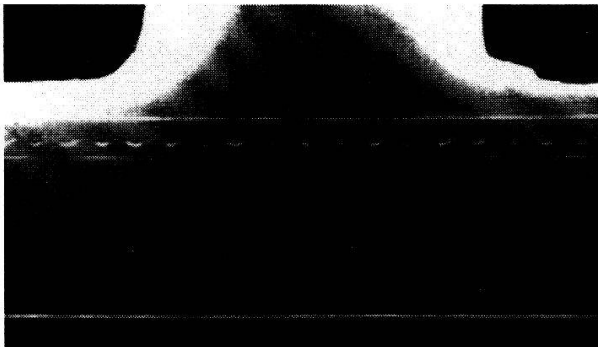
Figure 2: SEM photography of InGaAs QWW in a waveguide. Distance between two adjacent wires is 180 nm
