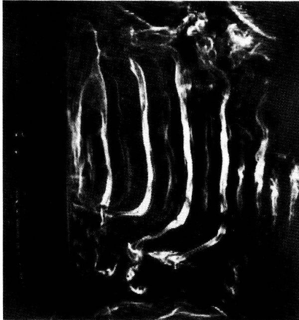
Fig. 1: Flow visualization of the wake behind the delta-shape body ( x - z -plane) at Re=100 . Here parallel shedding is obtained ( \Theta = 0^\circ ). The flow is from left to right
