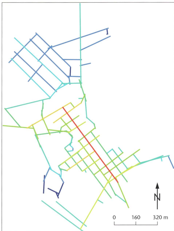
Abb. 6: Strassennetzwerk von Augusta Raurica. Axial Analysis, Integration (HH, n-streets = 98), UCL Depthmap Version 10.14.00b. M. 1:16 000.
