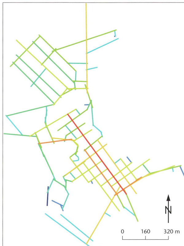
Abb. 7: Strassennetzwerk von Augusta Raurica. Axial Analysis, Integration (Radius = 2, n-streets = 98), UCL Depthmap Version 10.14.00b. M. 1:16 000.
