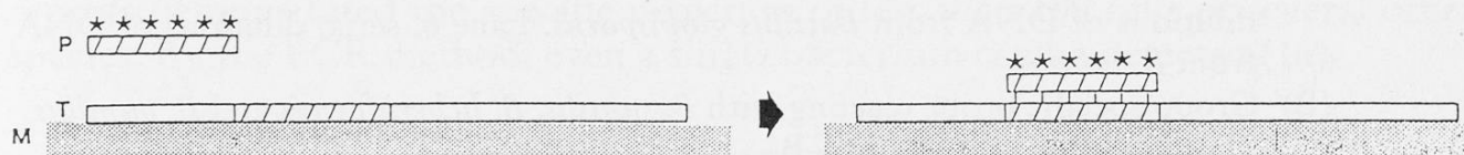
Fig. 2. Scheme of filter hybridization. H, hybrid; M, membrane; P, probe (asterisks indicate label); I, immobilized target nucleic acid
