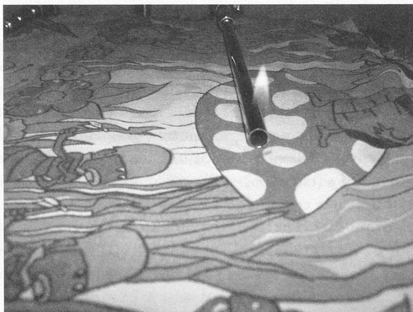
Picture 1 Duvet cover being tested with a small open flame according to EN 12952 parts 3 & 4
