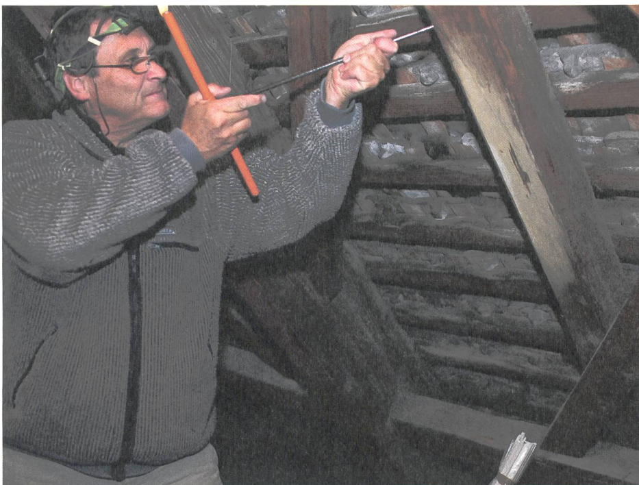
Sampling for dendrochronological analysis of roof truss.
