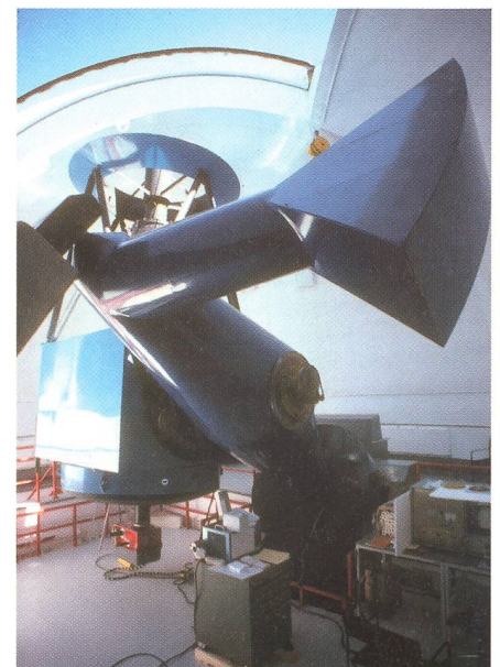
Fig. 15: P3 photometer attached to the Spanish 1.5 m telescope at the Calar Alto Observatory of the MAX PLANCK Gesellschaft, in Spain (photo: 1979).
