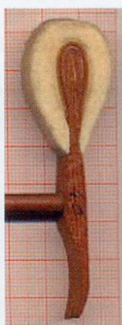
Illustration 24. Hammer for c 2 , grand piano no. 14,000 by Pleyel et Cie, Paris July 1847 (RA) (private collection, France; this serial number was provided by the owner) (Author's note: No. 14,000 is listed in LA as "piano droit 1/2 oblique": the nearest grand pianos to this are no's 14,043-14,050, 14,068-70 all "petit patron" or 14,062-66 "grand patron")
