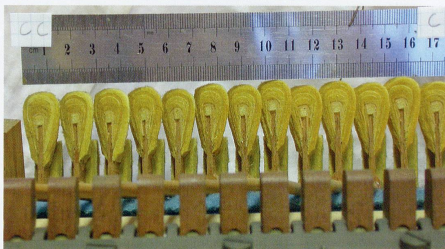
Illustration 15. Bass hammers, square piano no. 7,872 by Pleyel et Cie., Paris October 1839 (RA) (private collection, France)
