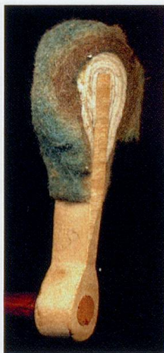
Illustration 9. Hammer from a square piano, probably by Pape, Paris c. 1835 (private collection, France)
