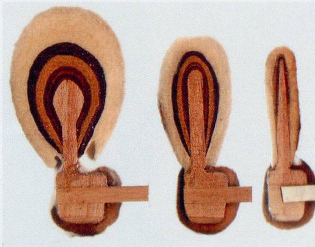
Illustration 26. Hammers for AAA, a 1 , a 4 , grand piano no. 9,772 by Erard & Co. London 1866 (Finchcocks Collection, England)
