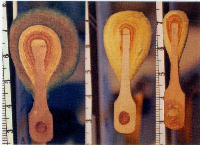
Illustration 7. Hammers for CC, c^2 , e^4 , square piano no. 13,107 by Sébastien & Pierre Erard, Paris 1834 (private collection, Switzerland)
