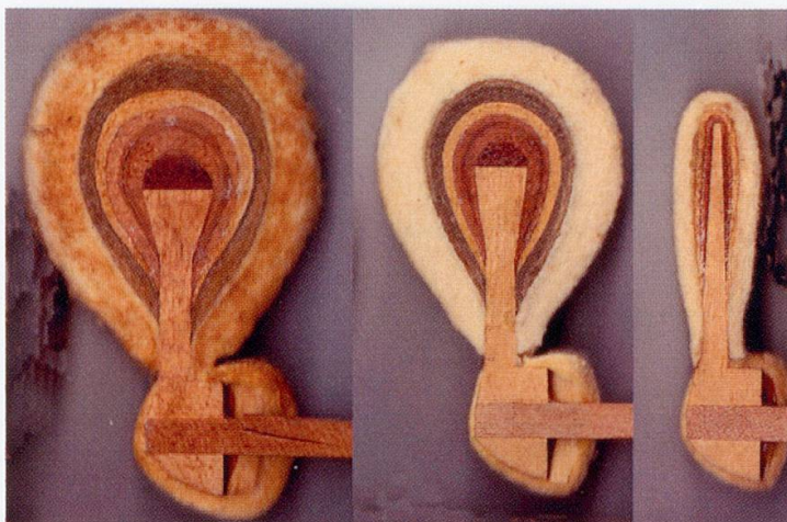
Illustration 19. Hammers for CC, c^1 , g^4 , grand piano no. 15,700 by Erard, Paris December 1842 (sold 2nd February 1843, Mon. Laurent, Namur) (private collection, Switzerland)
