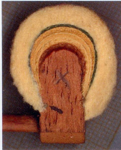
Illustration 11. Hammer for FF, pianino no. 5,998 by Pleyel et Cie., Paris October 1837 (RA) (RC November M. Henniquin (?), Paris) (private collection, France)
