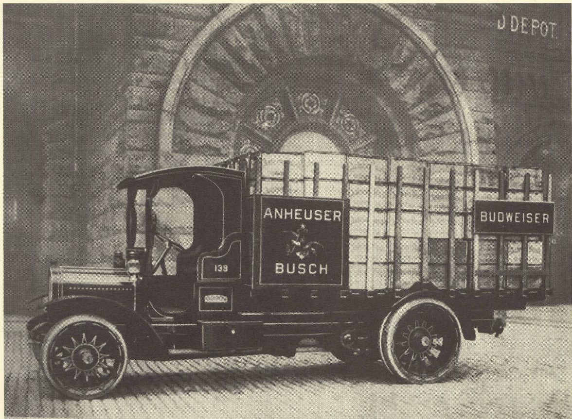
SAURER Truck used by Anheuser-Busch Company, St. Louis, Mo. With about eighty-five per cent of the load-weight on the rear axle, SAURER design gives the engine utmost protection and saves general wear and tear.
