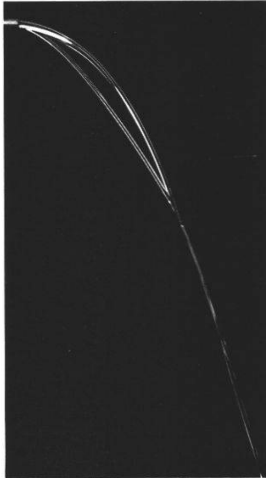
Fig. 4. Jet laminaire, Re = 260 .
