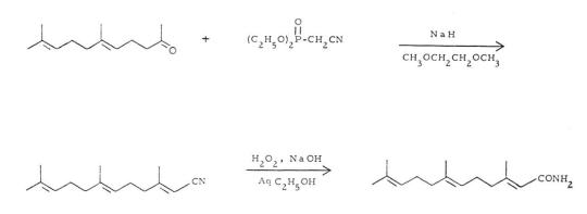
cyanomethylphosphonate gave the farnesonitrile. Hydrolysis of this in aqueous ethanol gave the desired unsubstituted farnesamide which could be converted to the 10,11-epoxy derivative by peracid.
