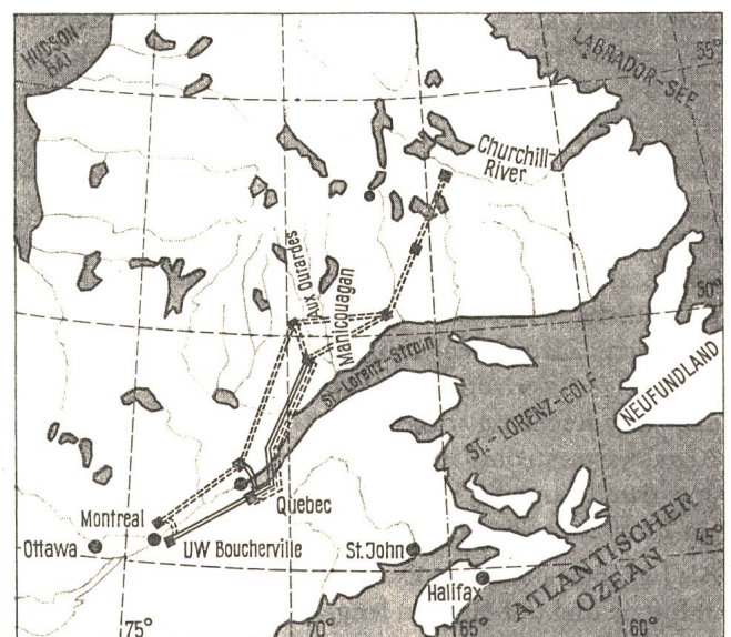
Fig. 7 Das 735-kV-Netz der Quebec Hydro-Electric Commission [34]
