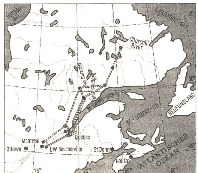
Fig. 7 Das 735-kV-Netz der Quebec Hydro-Electric Commission [34]
