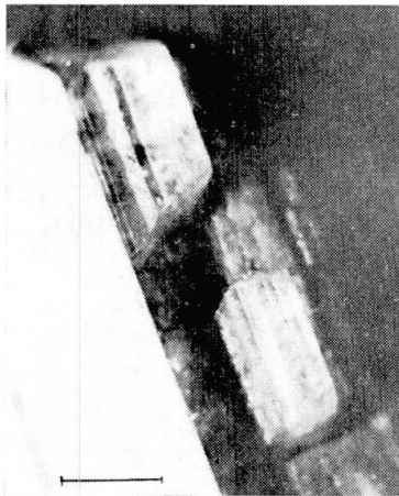
Fig. 5. Idiomorphic albite crystals with "staircase faces". The uniform albite layer on (010) with idiomorphic outlines towards (+a) is also visible. (5 mm on the photo = 1 mm.)
