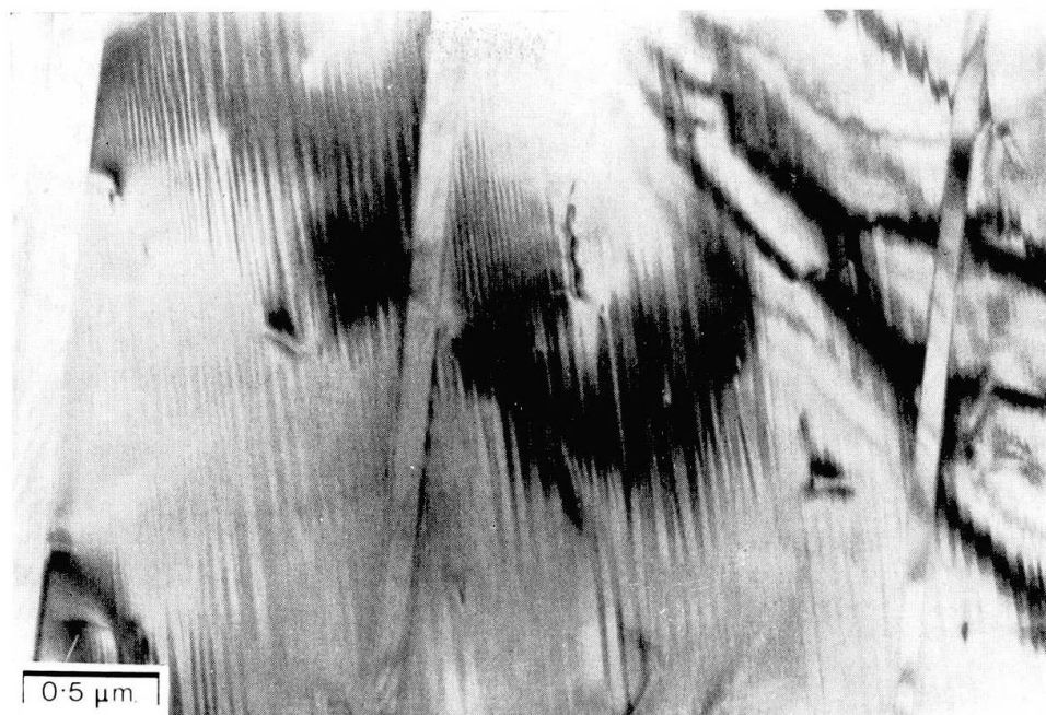
Fig. 5. 100 kV electron micrograph showing the variation in periodicity of the exsolution lamellae and three Albite twins (approximately vertical). The wavelength of the exsolution varies from 20 to 80 nm.
