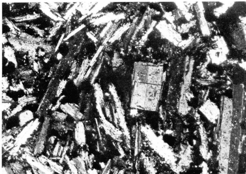
Fig. 16 Albite phenocryst in hematite spilite showing combination of Albite and Ala-A twinning laws. (L = 1.30 mm, with analyser)
