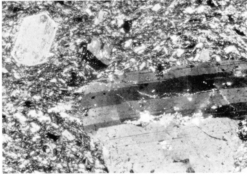
Fig. 13 Keratophyre. Phenocrysts of albite showing normal twinning, embedded in a felsitic matrix. Inclusion zoning is also seen. (L = 3.27 mm, with analyser)
