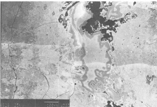
Fig. 7 SEM, BSE image, photomicrograph of sample 9: Penecontemporaneous braunite (br) and hollandite (hol) as principal manganese constituents, with pore-filling colloform hollandite and pyrolusite (pyr).
