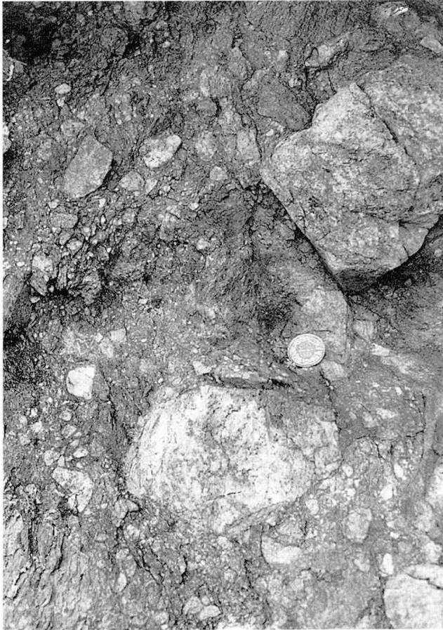
Fig. 5 Cataclastic fault breccia, derived from granitic/gneissic Tasna basement. Clasts of granite and gneiss, both angular and slightly rounded, "float" in a chlorite-rich, cataclastic matrix. This outcrop is about 15 meters below the basement-cover contact, southeast of Piz Clünas (coord. 814 500 / 189 200). Compare figure 4a. Diameter of coin is 2.7 cm.
