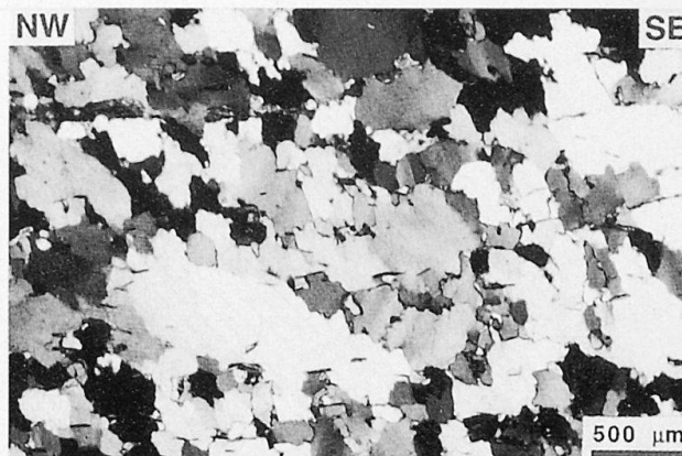
Fig. 3 Quartz microstructures from D_1 with grain boundary migration leading to oblique grain shape.
