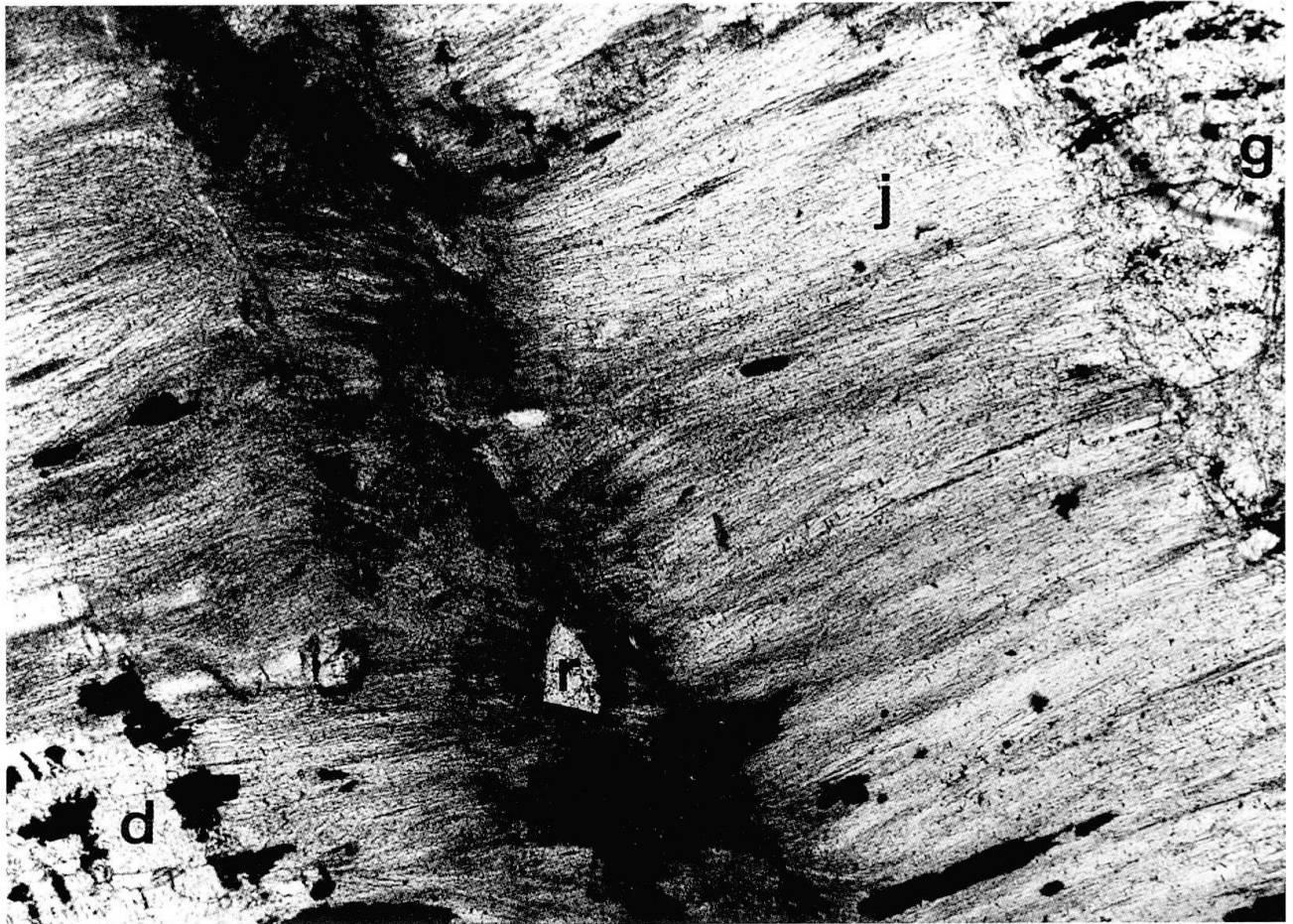
Fig. 1 Microphotograph of a johnninesite veinlet. j = johnninesite, r = roméite, d = dolomite (belongs to the veinlet), g = embedding ore, consisting mostly of dolomite, hematite, jacobsite, and manganian muscovite. Transmitted light, field of view 1.25 \times 0.92 mm.
