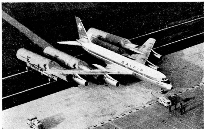
Swissair's new detuner installation is seen here connected to the engines of Coronado HB-ICH operated by Balair.
