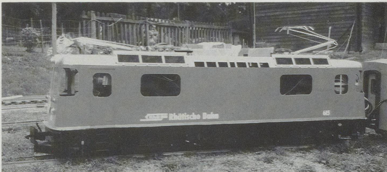
RhB in Devon. 1/5th size (7 1/4" gauge) model of Ge4/4/II No 615 built by Pfeifferbahn for Alan Kitchenside's Gorse Blossom Railway, nr Newton Abbott. 3x1HP 12V motors, electronic control, rheostatic and air brakes plus 500kg of batteries in the baggage car! Photo Don Fifer
