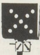
8. Shunting is forbidden. The track protected by this signal must be cleared immediately and kept free.
