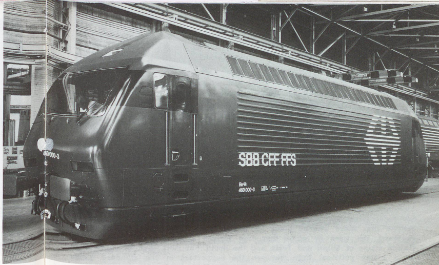
Above : The body of the first Re4/4 460 class locomotive at SLM, prior to despatch to ABB for the electrical and running gear. Photo SLM
