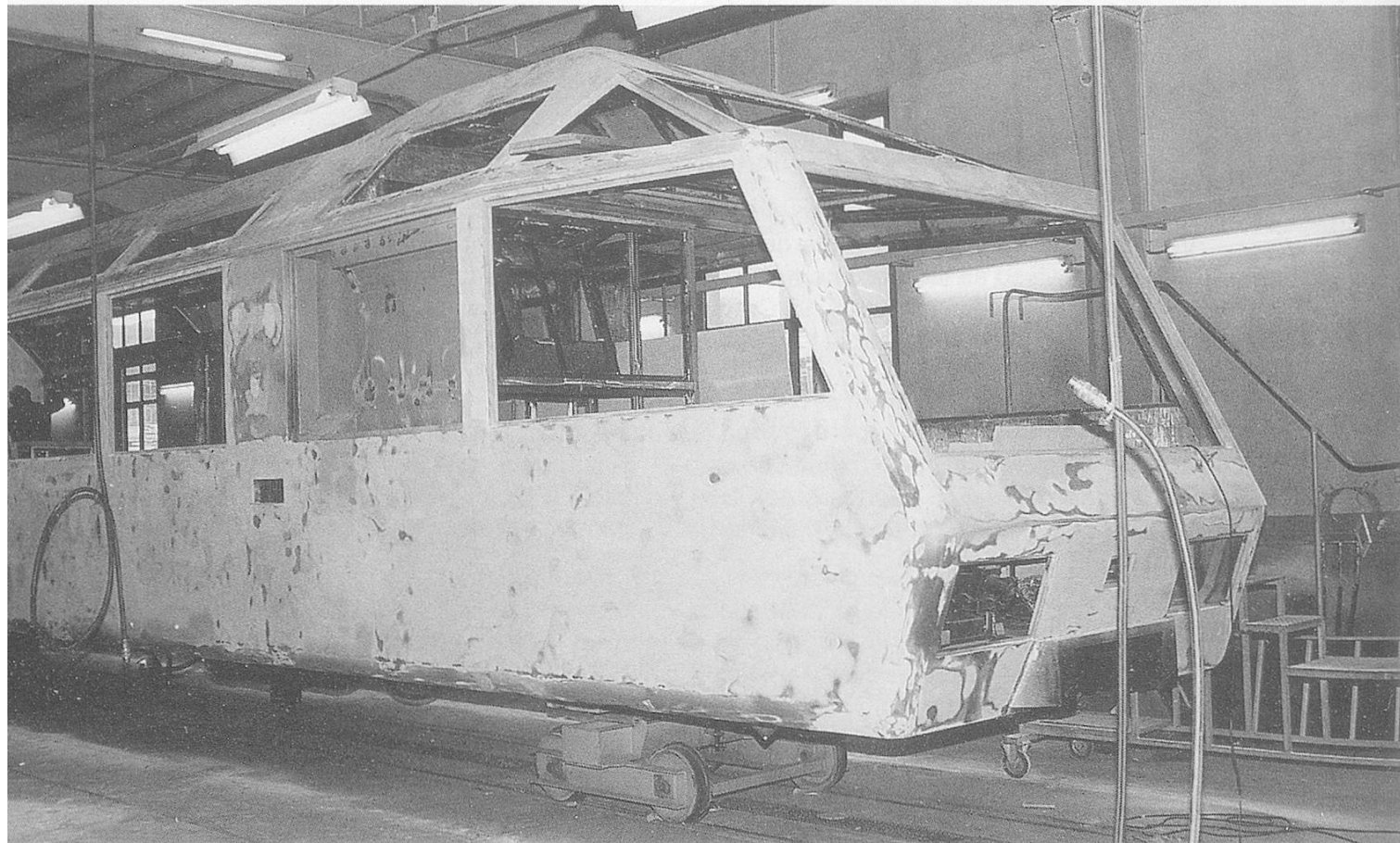
Below: The Driving trailer in the Chernerx works undergoing a complete refurbish, notice the raised driving position.
