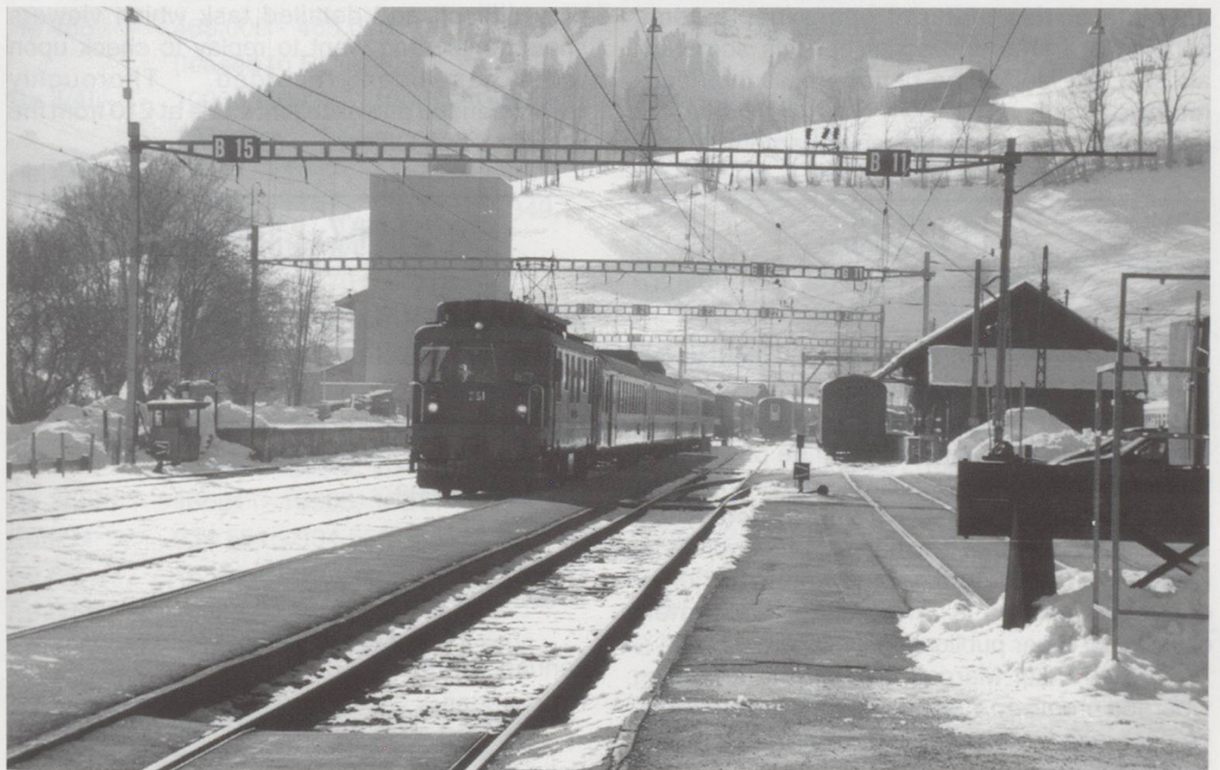
Zweisimmen: BLS Ae4/4 No.251, brought out of storage due to locomotive shortages, works a Zweisimmen to Interlaken express. Photo: Peter Bowen
