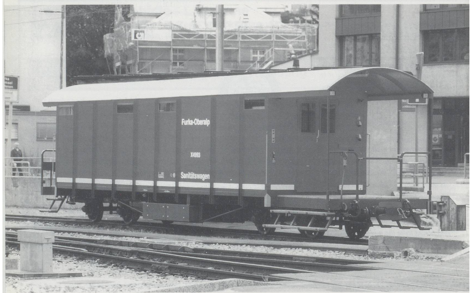
Below: A new tunnel vehicle in case of accidents in the Furka Basis tunnel this one is to be kept at Oberwald supplementing the one already based at Realp.
