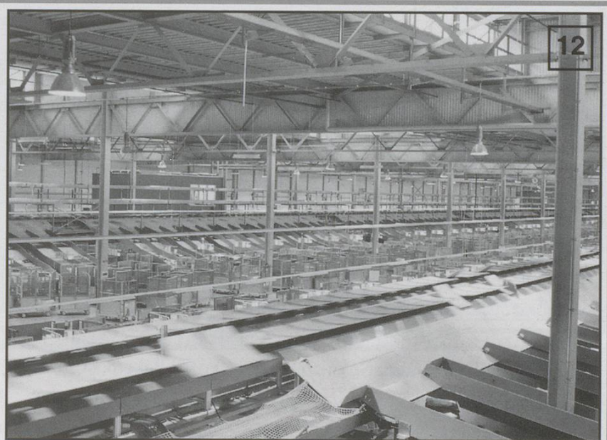
In the huge 1,000. ft. long hall, the parcels travel on continuous conveyors with tipping platforms, which lead into one of the 337 destination bins.
