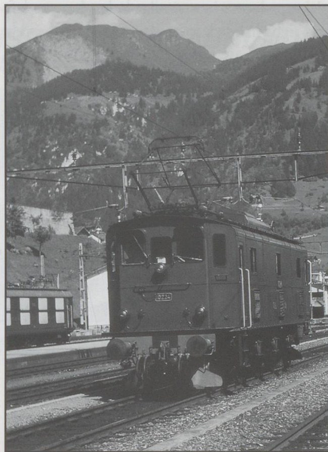
Of the several CFF classes fitted with Sécheron drive, the Ae 3/5 class was the smallest, its members sometimes being known as "Baby Sécherons". 26 of them were built between 1922 and 1925 by SLM and SAAS and spent most of their lives working in the French-speaking parts of the country. During the 1960s, 10218 10226 were modified to work car trains through the Gotthard and Simplon tunnels and one of these, 10224, was photographed at Airolo in the summer of 1967.
