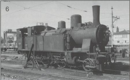
The 2-8-0, 2705, was one of a class of 32 locos built by SLM between 1904 and 1906 and withdrawn 1931 - 1963. They weighed 112 tons and were authorised up to 65 km/h.
