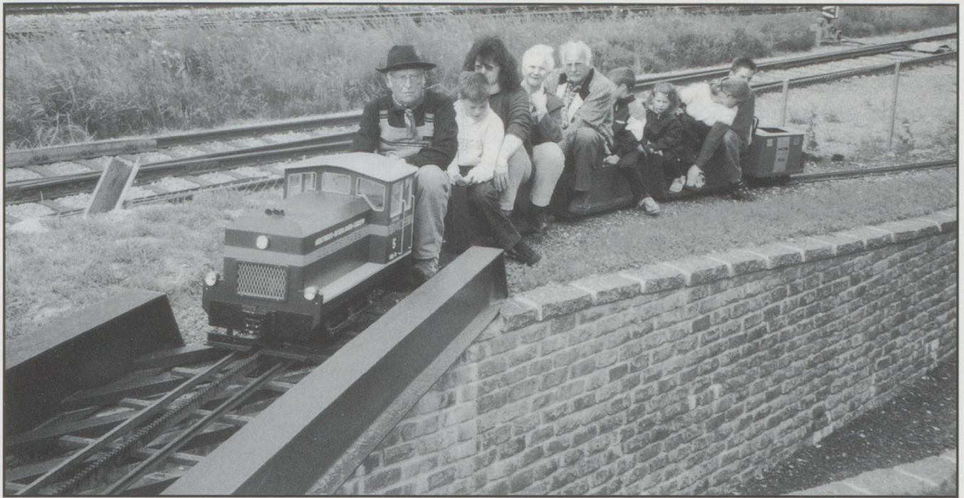
A 7 1/4" gauge model of a Diesel Hydraulic climbs the 100% rack track with quite a load. Battery-electric powered with electronic speed control. June 2000. Photo: Bernard Fenton
