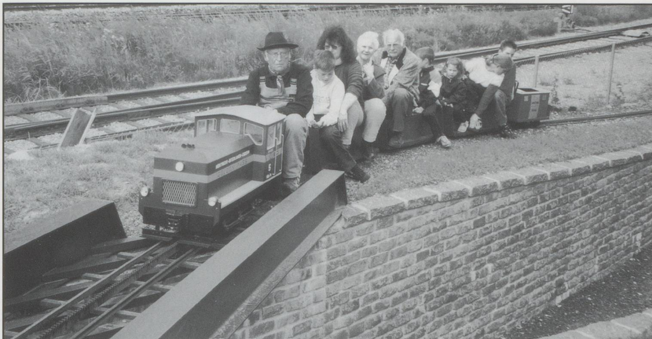
A 7 1/4" gauge model of a Diesel Hydraulic climbs the 100‰ rack track with quite a load. Battery-electric powered with electronic speed control. June 2000.
