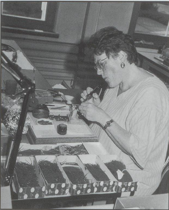
All electrical connection leads are precut to size and tinned, prior to being fitted by hand.
