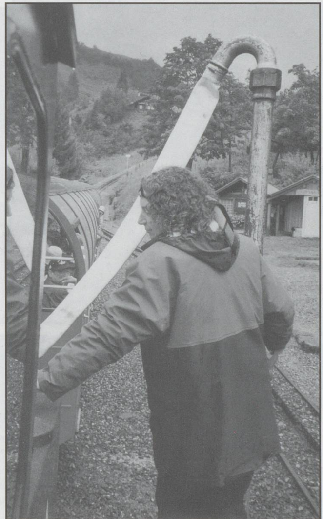
Watering the loco as viewed from the footplate.
