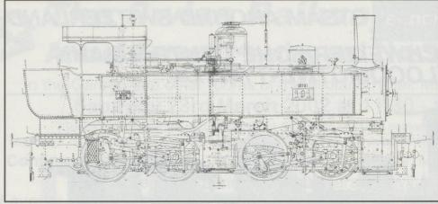
pressure. The two 1 280 mm diameter driving wheels in each unit had a wheelbase of 1,900 mm giving the locomotive a wheelbase length of 6,200 mm and a total overall length of 11,517 mm. Two leaf springs mounted under the smoke box kept the front unit aligned.
