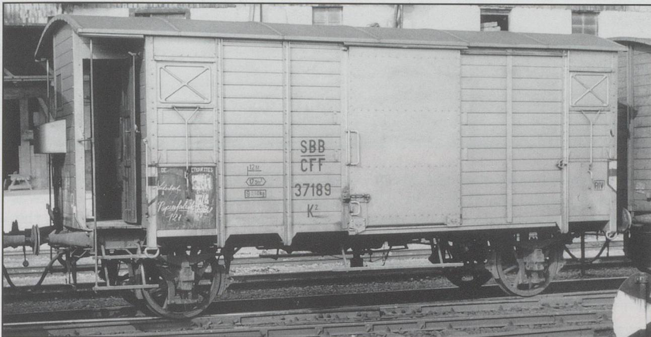
More K<sup>2</sup> vans were built than any other type of goods vehicle in Switzerland. This example, 37189, was photographed at Zürich in 1955. Instead of the usual grey livery, this vehicle had been painted white. Photograph courtesy *Eisenbahn Amateur*.
