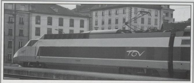
As Geneva station is directly connected to one of the French electric current systems (the 1500 Volt DC one) the service to Paris is operated by the normal French 2-current TGV sets. Such a set is seen here in its new blue livery and with the new logo. Now turn the page upside down and look again at the logo: it looks like a SNAIL, with a house on it's back....
