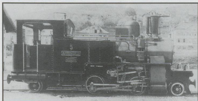
4.2.6 - First locomotive built to the Winterthur system and delivered to the Appenzellbahn.
