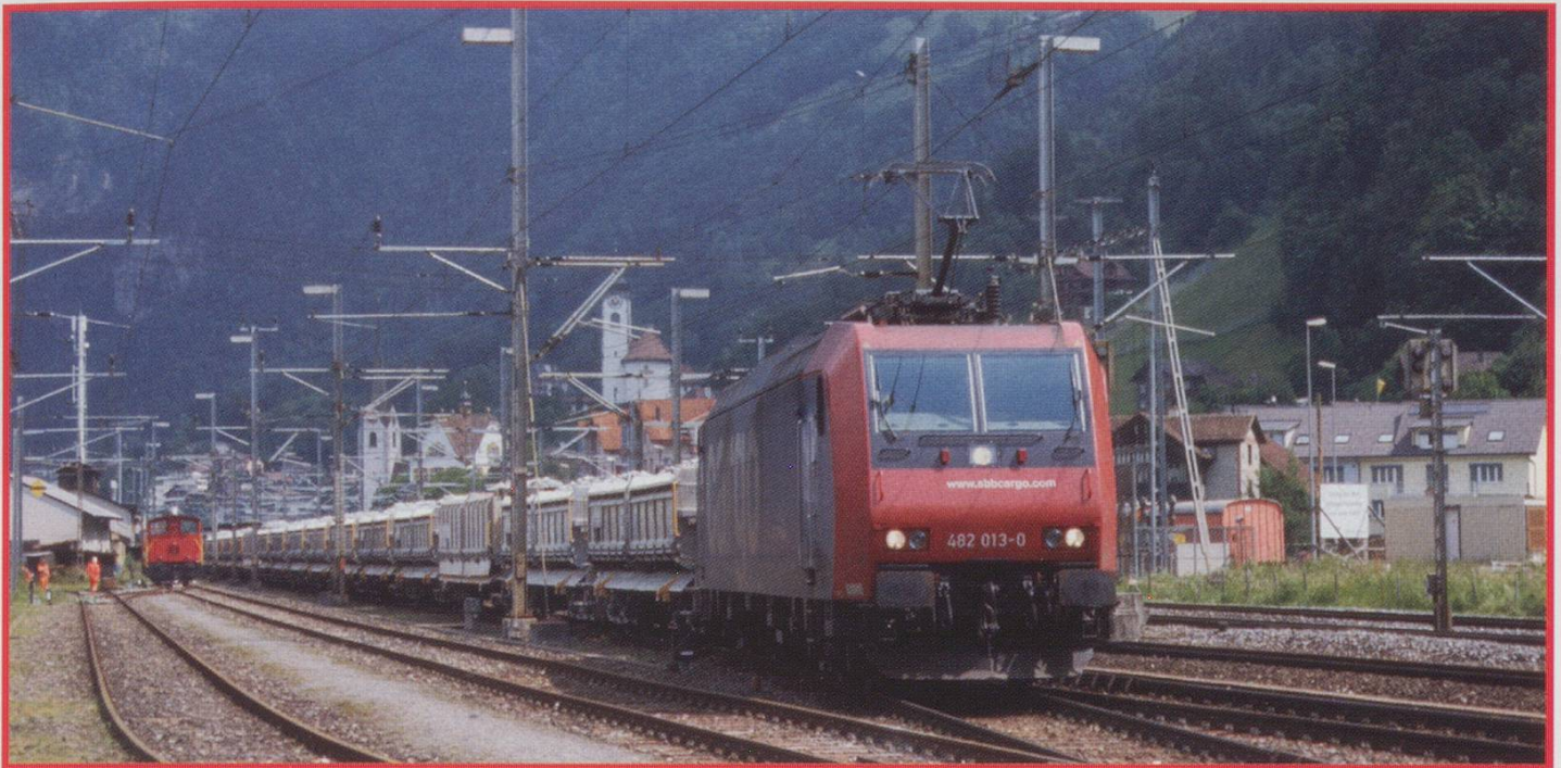
482013 moving forward before reversing its train over the level crossing. The on-board videocam is just above the handrails on the side of the loco.
