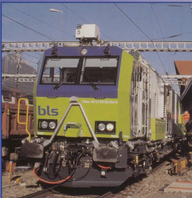
BOTTOM LEFT: The front of the business end; the white box on top is a foam sprayer – the train carries 1600 litres of foam and 52,000 litres of water. The most successful way to extinguish a fire is to spray the water in a fine mist; apparently the effect is quite dramatic. The control in the leading cab is designed to withstand extreme temperatures and air is supplied from the pumps.
