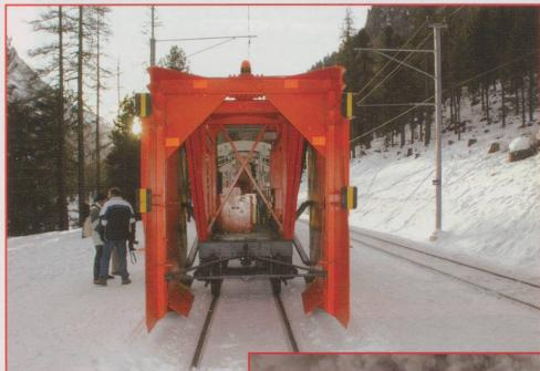
This snow spreader is used on the RhB to assist in winter clearance work after a heavy snow fall. The vehicle has movable wings and is used to set the width of the path through the snow. It is pulled at the end of a works train to cut and funnel the snow to an area where it can be blown with the snow blower.
