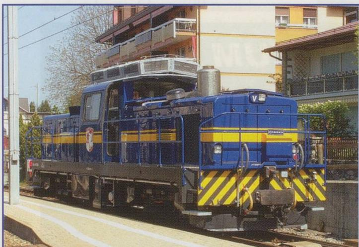
Monday 5th May saw the roll-out of MOB diesel-electric locomotive Gm4/4 No.2004 *Albeuve* after a major overhaul. Built in France by Gaston Moysse of La Corneuve, this loco entered service in 1982, six years after its sister No. 2003 *Montbovon*. These powerful diesels are used for works trains and can also haul passenger stock if there is a problem with the catenary.
