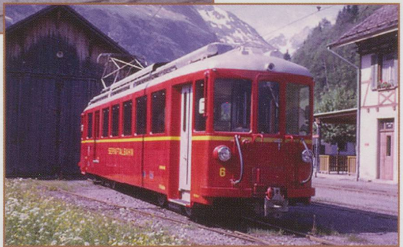
SeTB No. 6 is a CFe 4/4 built by SWS and MFO in 1949 and still at work with the Stern & Hafferl organisation on the Achensee line in Austria. The picture is also taken around 1969 at Elm station by Peter Sutter. The red livery comes from the colour of the regional arms Glarus/Glaris/Glarona with the Saint Fridolin in black on the red ground.
