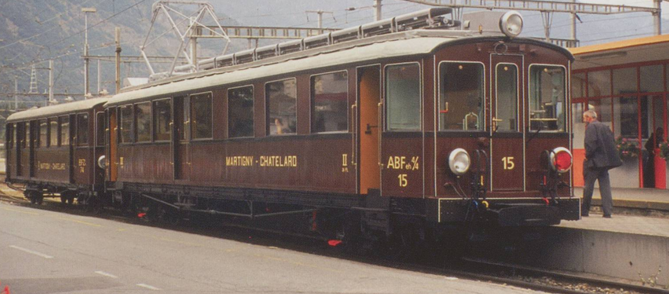
When running trips from Martigny to Vernayaz on the open day on 8 September 2001, automotrice No.15 was classified as ABFeh 4/4, although in publicity for this year's Le Valais en fête she is described as BCFeh. ALL PHOTOS: Michael Farr
