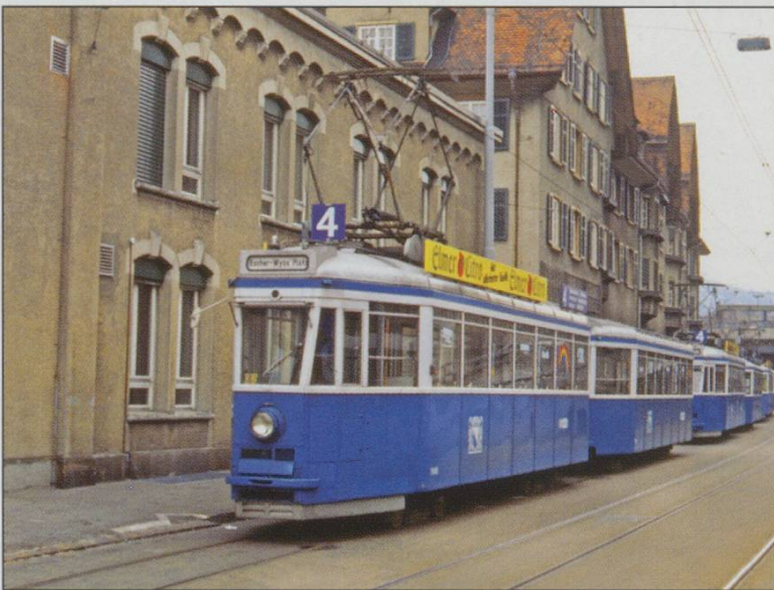
TOP: VBZ "Karpfen" bogie cars 1419+779 at Irchel. Note the odd central window on the leading car designed for an abortive plan to insert an offside door for running in tunnels with central platforms, 08/12/1985.
